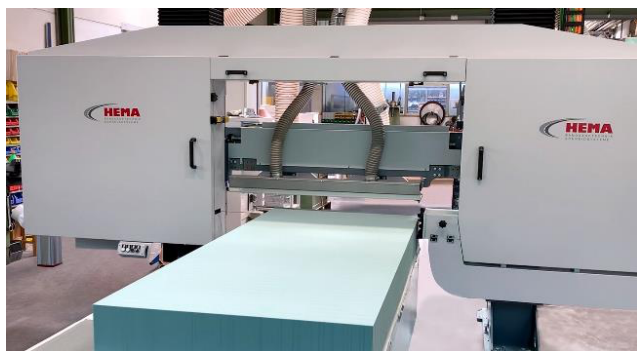
Fig. 2: HEMA CoreCutter 900 for cutting PET rigid foam
