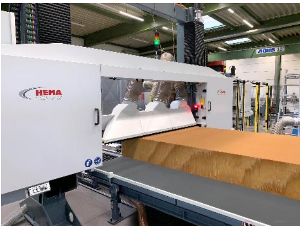
Fig. 1: HEMA CoreCutter 900 for cutting aramid honeycomb blocks
